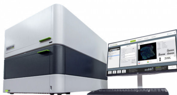
Figure 1. The GeoMx DSP enables spatial analysis of RNA and protein in tissue slides. (Source: NanoString)
