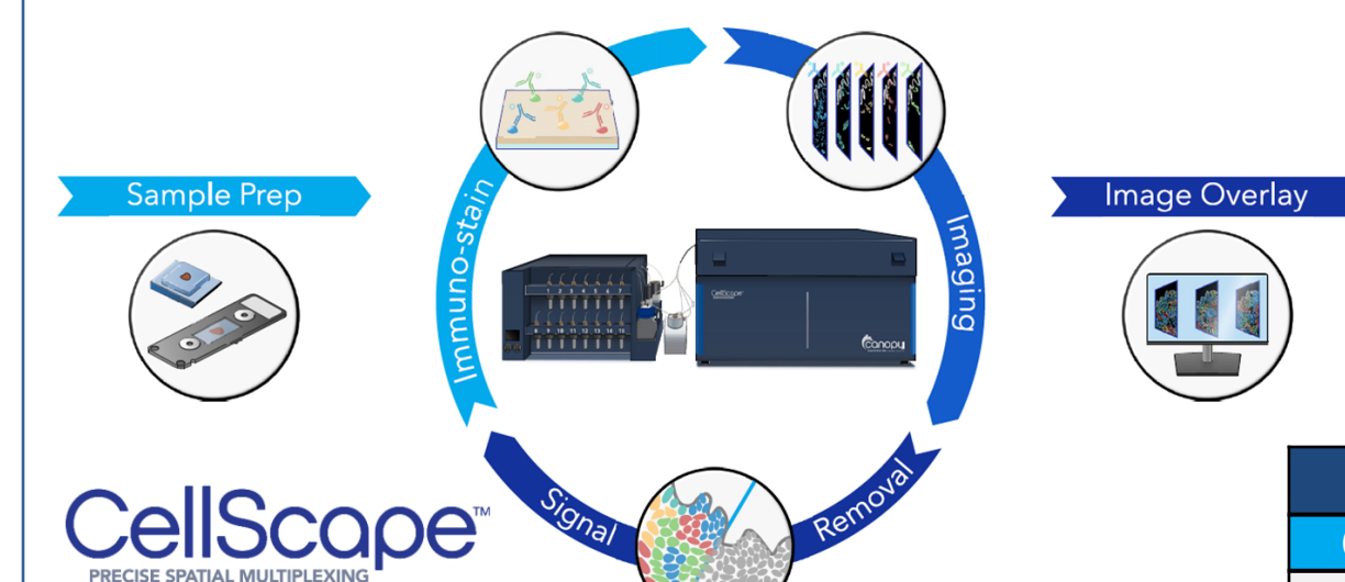
Figure 1. ChipCytometry workflow. After sample preparation, the ChipCytometry workflow consists of successive rounds of immuno-staining, imaging, and signal removal to profile virtually unlimited number of protein targets. An image overlay of each marker in the assay is created by aligning each channel to a reference channel. The process is fully automated with CellScope, the next-generation instrument for precise spatial multiplexing.
