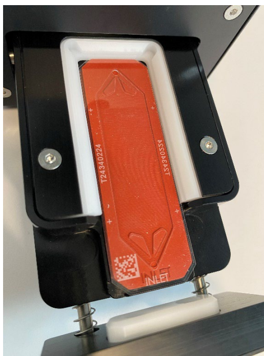
Figure 3. Placing the WSIC coverslip correctly onto the silicone pad of the Slide Assembly Tool.
